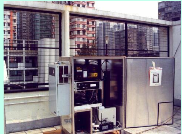
tapered element oscillating microbalance - continuous RSP
