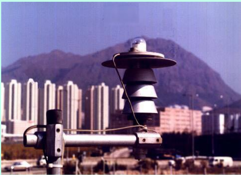
Solar radiation detector
